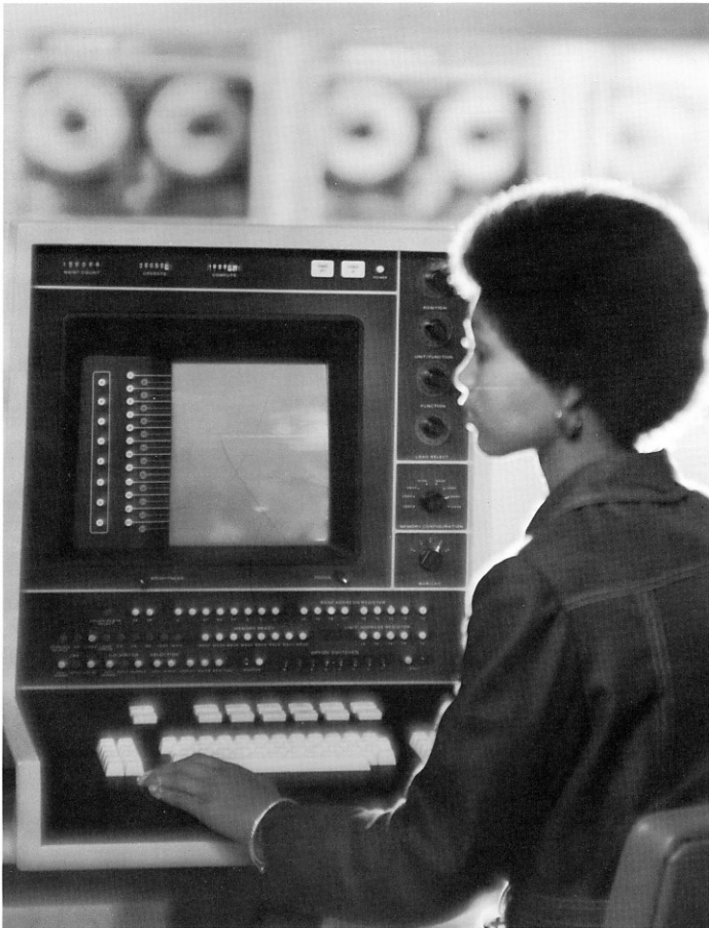
As a standard feature, NCR Century 300 includes an integrated CRT console for fast operator/system communication.
